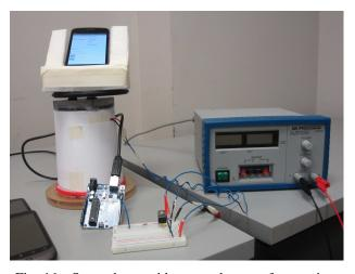
Fig. 16: Smartphone with external motor for rotation.
