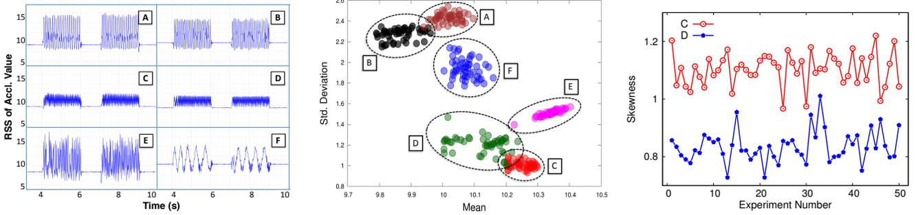
Fig. 4: Accelerometer responses of 6 chips for the same stimulation: (a) Using *Root Sum Square* (RSS) of the three axes over time offers some differentiation among chips; (b) Clustering on 2 dimensions – RSS mean and deviation – improves separation; (c) Clusters that overlap with mean/deviation, separate out further using a *Skewness* feature.
