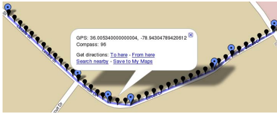
Fig. 2. Large blue icons marks the piecewise segments of the polyline, while black icons are computed intermediate points. Each location associated with the latitude, longitude and the angle from magnetic north.
