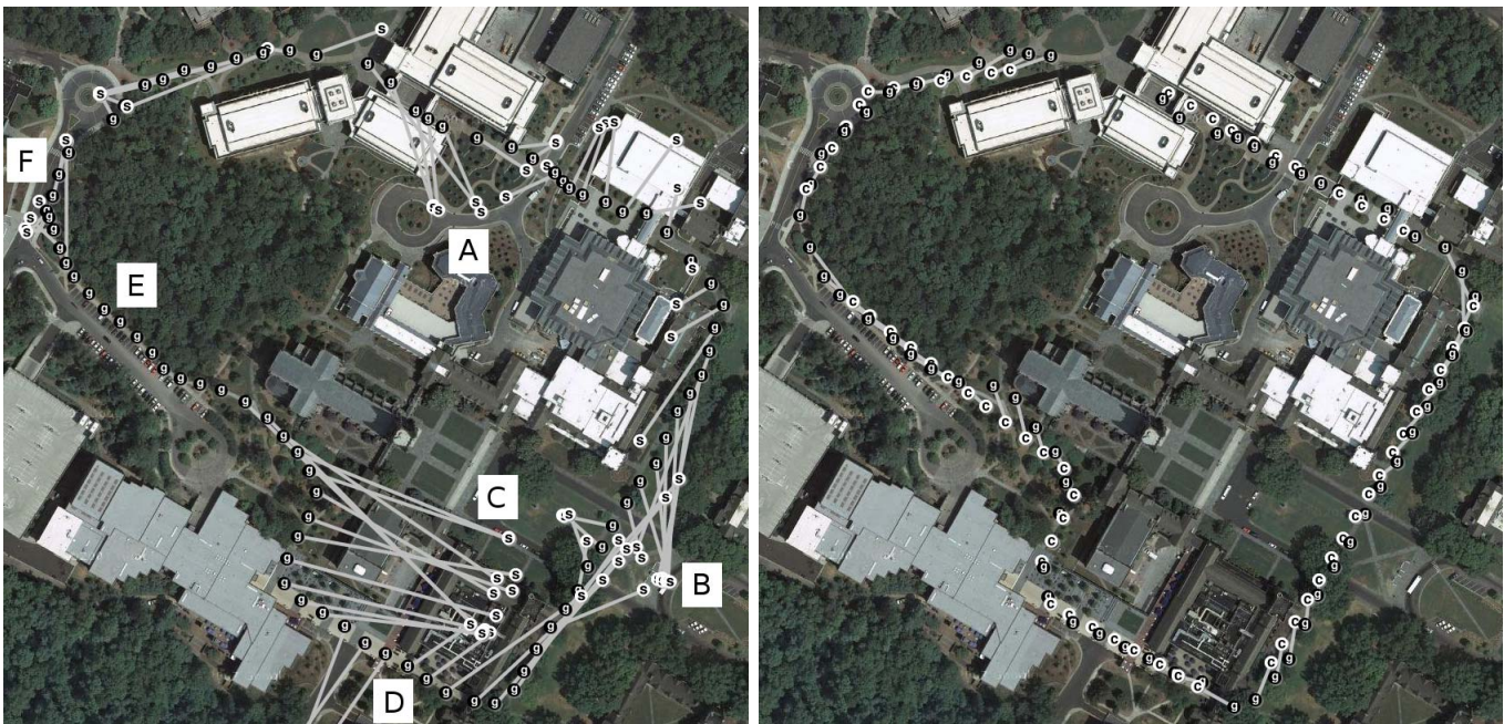
Fig. 13. Visualization of (a) Skyhook's and (b) CompAcc's performance in Duke campus. GPS locations shown by "g", Skyhook by "s", and CompAcc by "c". Straight lines joining s-g and c-g are a measure of the location errors. Some regions do not have a "s" value because Skyhook was unavailable there.
