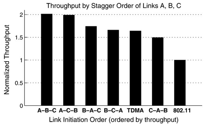
Fig. 13. Multiple Shuffle orders provide higher throughput than both TDMA and 802.11.
