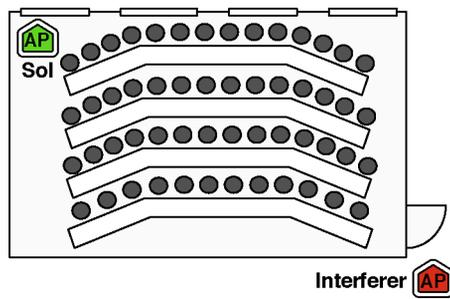
Fig. 17. Classroom environment with 54 seats. Leaving the AP and one client fixed, we tested with a client placed on the desk in front of each chair.
