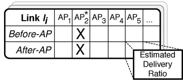
Fig. 8. Per-link data structure maintained at the controller for scheduling transmissions. AP<sub>2</sub> is the transmitter for link  $l_i$ .
