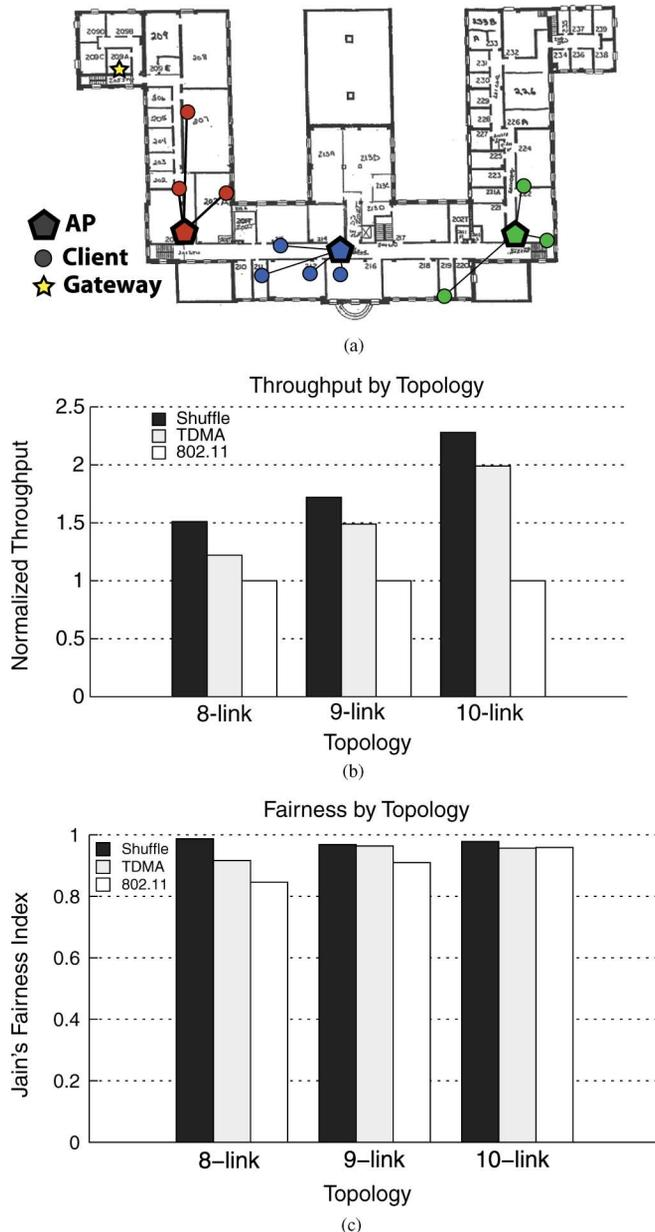
Fig. 15. (a) Example 10-link topology in our building. (b) Throughput and (c) fairness on entire Shuffle testbed.
