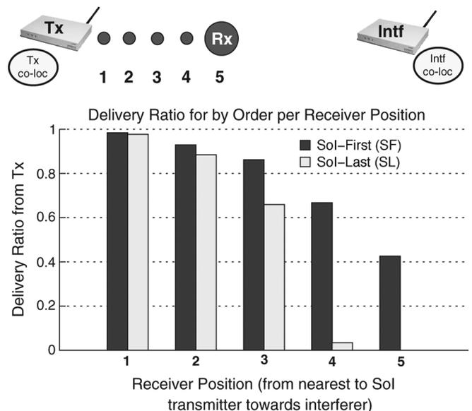
Fig. 5. Testbed confirms MIM capability. Rx receives from Tx (at five positions) in the presence of interference (Intf).
