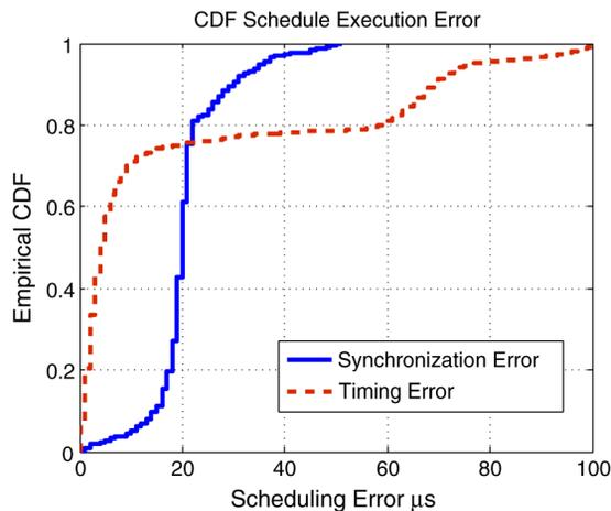
Fig. 11. AP-to-controller clock synchronization error and transmission deviation from the assigned schedule, relative to the local clock. AP and controller separated by approximately 20 m of CAT-5 cable, one switch, and one hub. Margin of error  $\leq 5 \mu s$ , attributable to 802.11 TSF inaccuracy.
