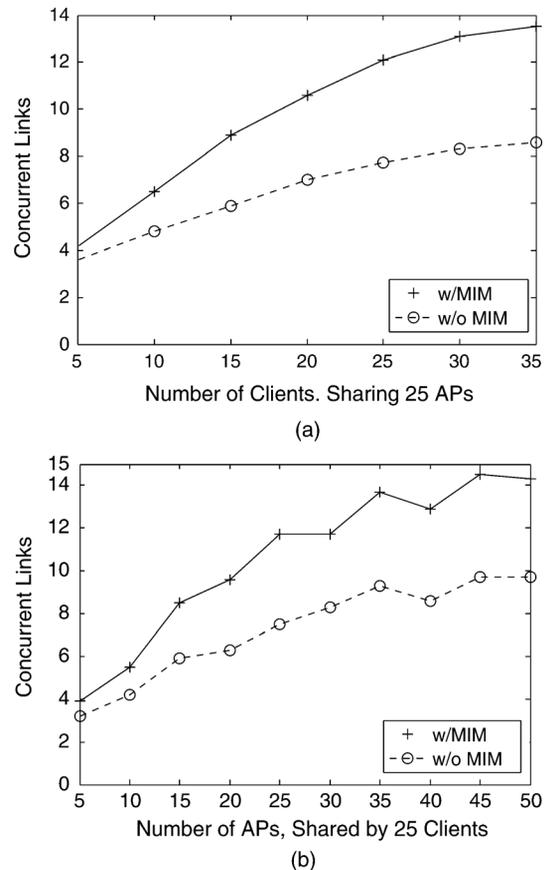
Fig. 6. MIM can provide large concurrency gains. These graphs show the number of links that can meet SINR requirements with and without MIM enabled. Gains improve with increasing network density. (a) Varying number of clients. (b) Varying number of APs.
