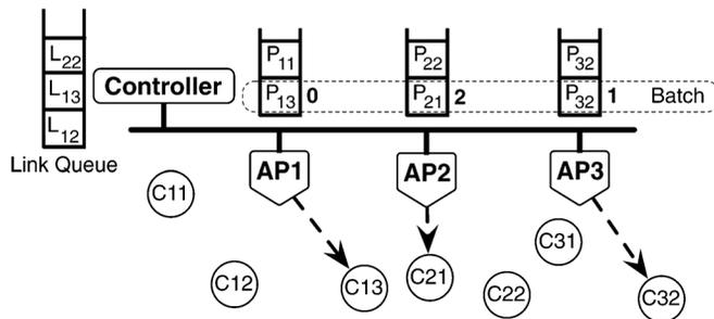
Fig. 10. Illustration of a scheduled batch of packets with the staggered transmission times. AP1 starts first, followed by AP3, then AP2.
