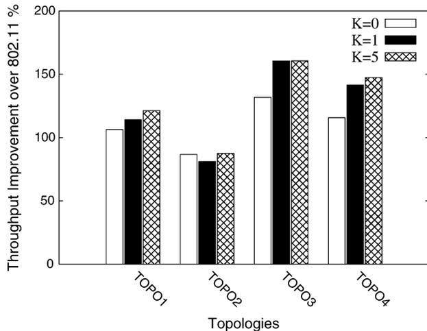
Fig. 20. Throughput improvement under different channel fading conditions. Shuffle performs well under Rayleigh and Ricean fading.
