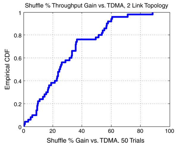
Fig. 16. Throughput for Shuffle versus TDMA using 802.11g with 6–54-Mbps rate control enabled.
