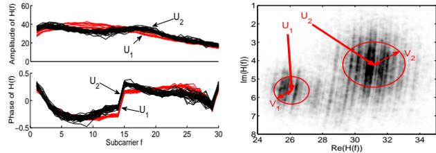
Figure 1: (a) The amplitudes and phases of the channel responses of 50 (out of 20000) packets sent over a link (we see two unique clusters,  $U_1$  and  $U_2$ ) (b) PDF of the complex value of the 20000 channel responses for a single subcarrier
